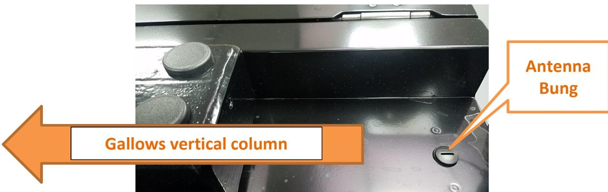
Top mounted displays supplied from July 2022 do not have a GPRS bung hole on the top face, therefore can be installed with the serial number label end facing away from the vertical gallows column where then viewable.
