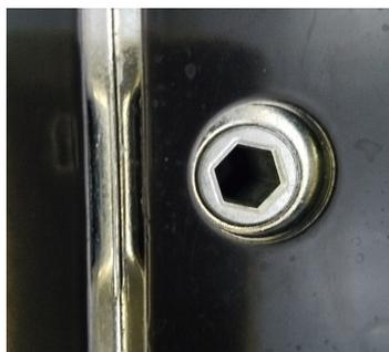
Display correctly closed (no gap at latch) ✓
